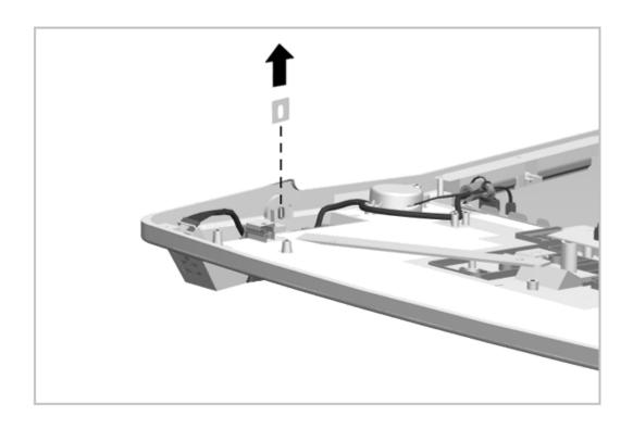
Figure 6-38. Removing the Security Lock Bracket
